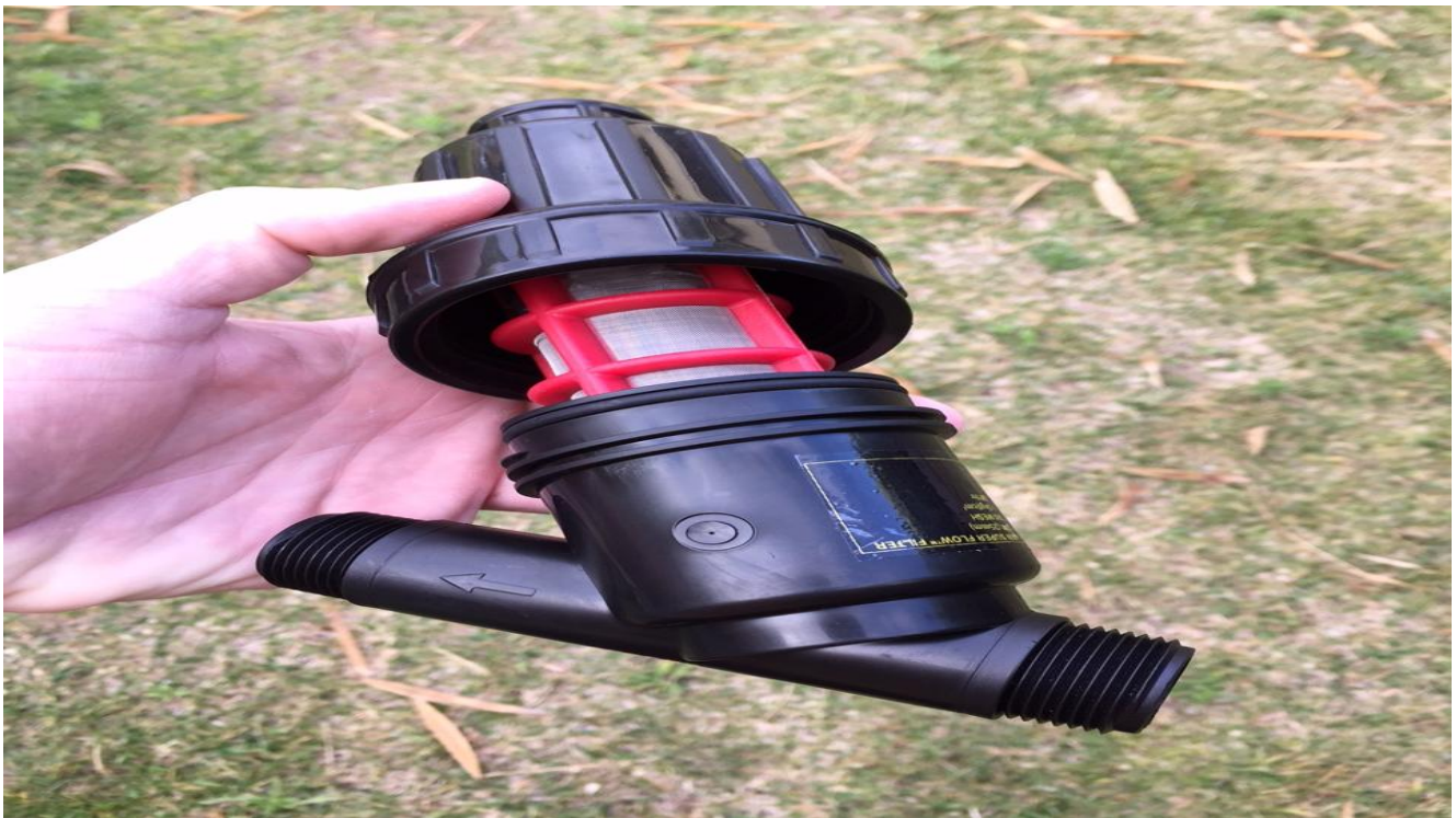
Figure 69: Filtration for Drip Irrigation Systems
